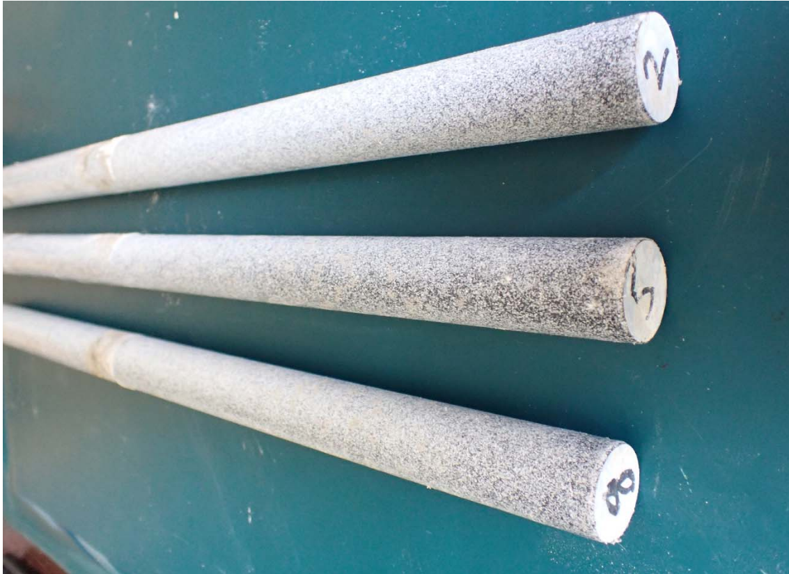
Picture 1: Tested dowels No. 2, No. 5 and No. 8 without damage or delamination of coating.
